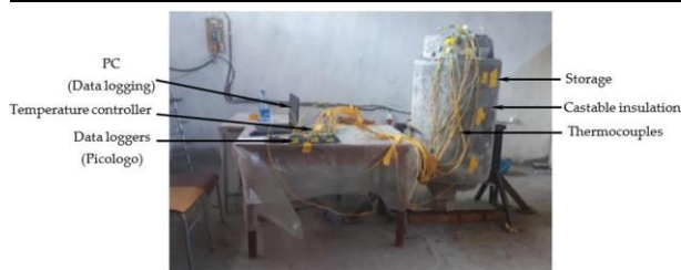
Figure 6: Experimental set up of the TES (Natural convection).
