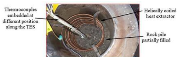
Figure 7: Internal part of the TES before fully filling the rock piles
