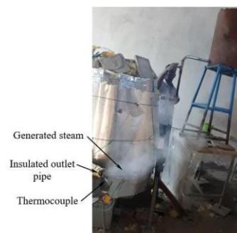
Figure 11: TES discharging with load using water.
