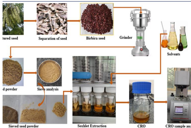
Fig. 1. General process flow diagram of CRO extraction by Soxhlet extractor.
