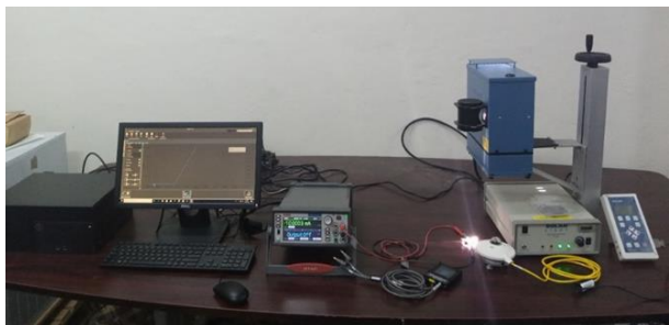
Figure 6. Setup of solar simulator and I-V measurement systems.
