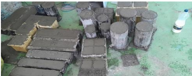
Figure 2. Concrete test samples for mechanical property determination.
